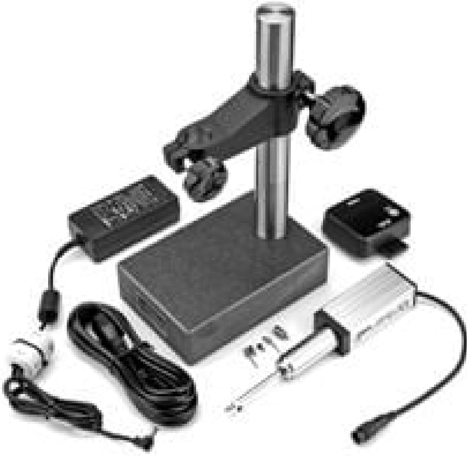
Nikon DIGIMCRO Digital Length Measuring System
