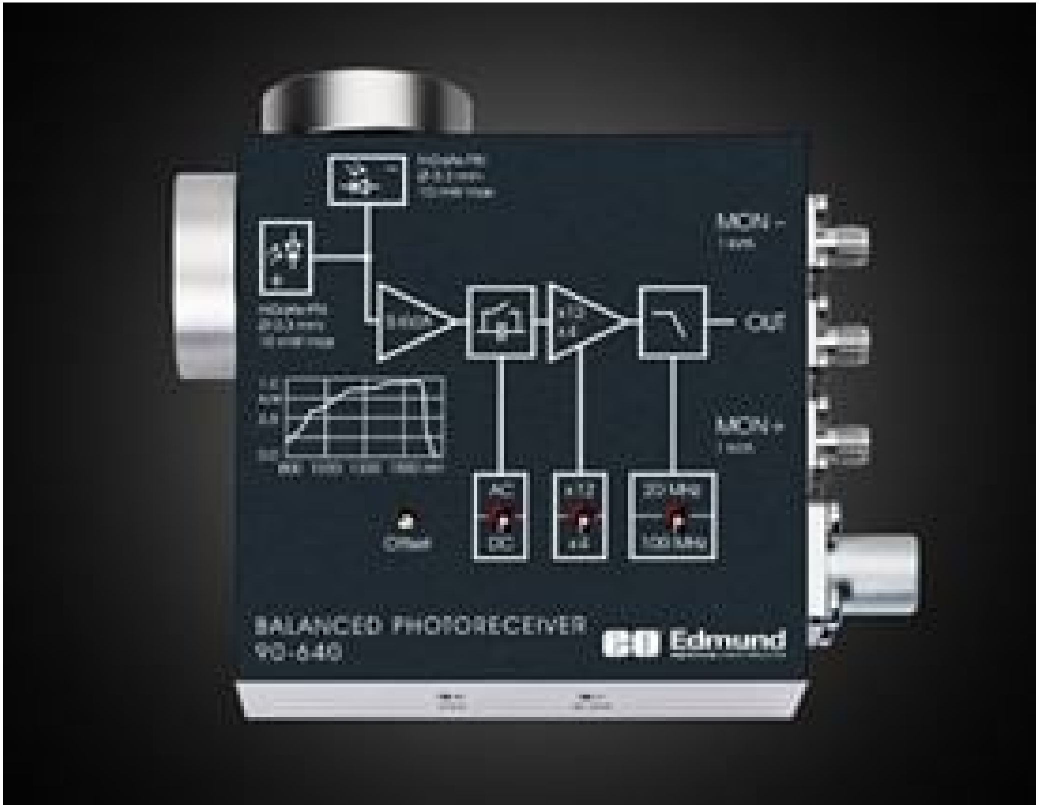
#90-640 InGaAs Free-Space Balanced Photoreceiver, 800-1700nm
