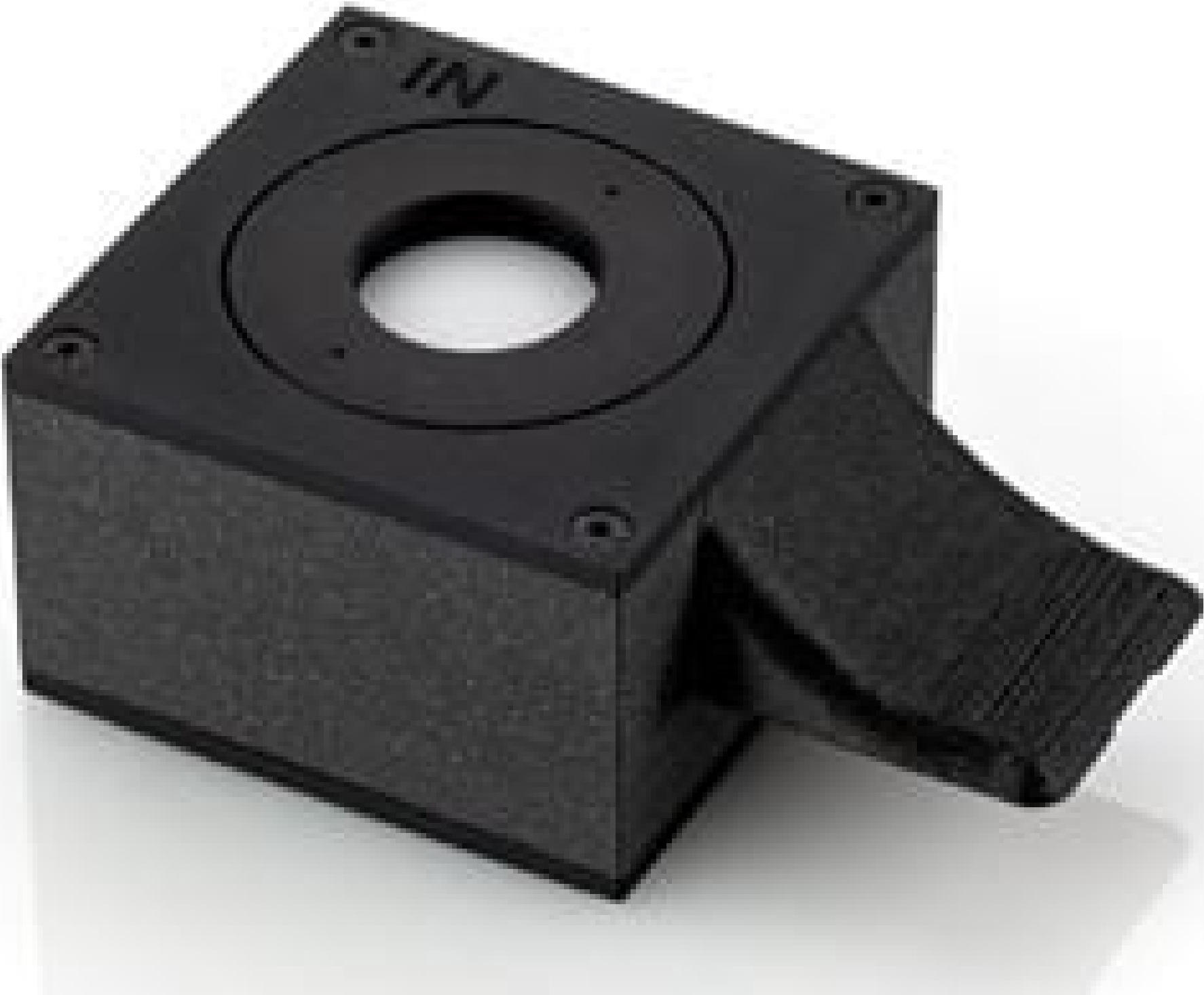
fNIRS Standard Phantom - IEC 80601-2-71
