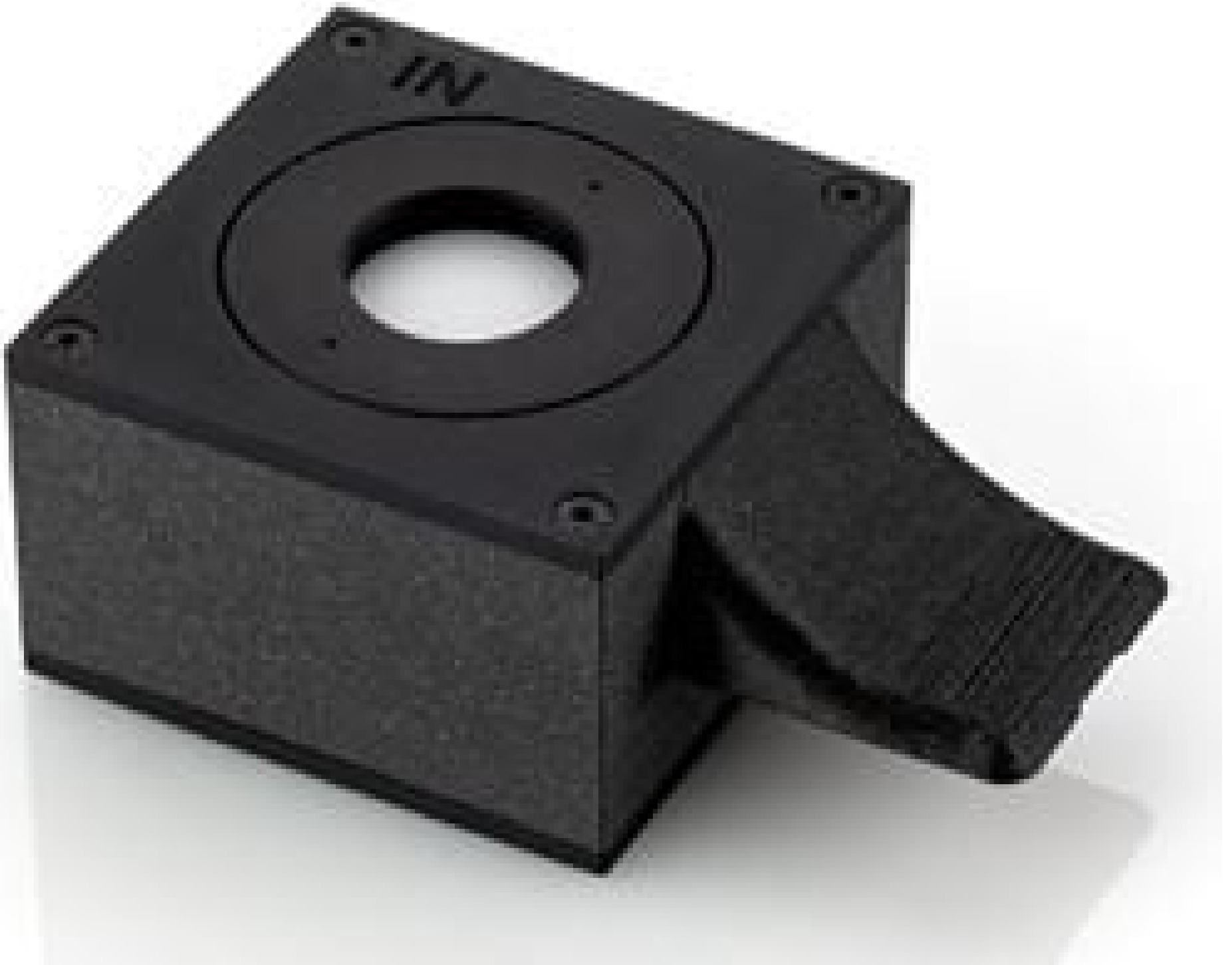
fNIRS Standard Phantom - IEC 80601-2-71
