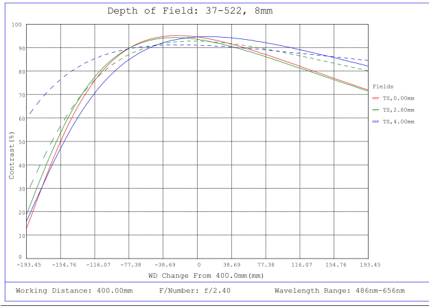
#37-522, 8mm FL, Liquid Lens M12 Lens, Depth of Field Plot, 400mm Working Distance, f2.4
