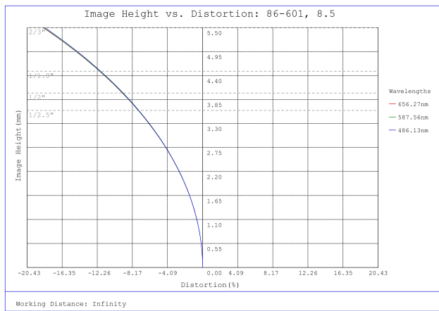
#86-601, 8.5mm, f/2.8 Ci Series Fixed Focal Length Lens, Distortion Plot
