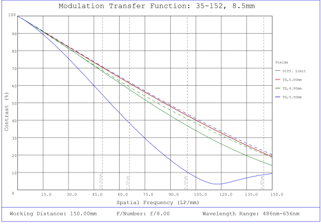
#35-152, 8.5mm, f/8.0, 75mm-∞ Primary WD, HRr Series Fixed Focal Length Lens, Modulated Transfer Function (MTF) Plot, 150mm Working Distance, f8
