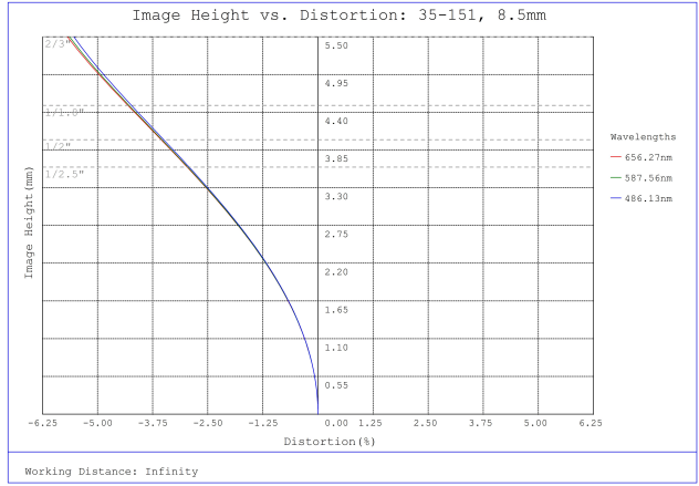
#35-151, 8.5mm, f/5.6, 75mm-∞ Primary WD, HRr Series Fixed Focal Length Lens, Distortion Plot
