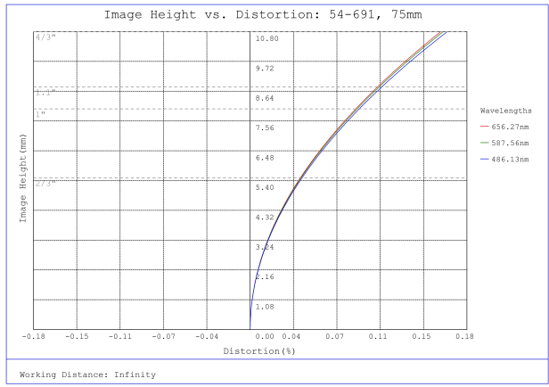
#54-691, 75mm DG Series Fixed Focal Length Lens, Distortion Plot
