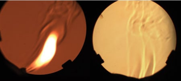
Flame Analysis using 6" Schlieren System
