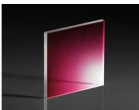
#23-374 - 50mm Sq., 1mm Thick, MgF 2 Coated λ/4 N-BK7 Window
