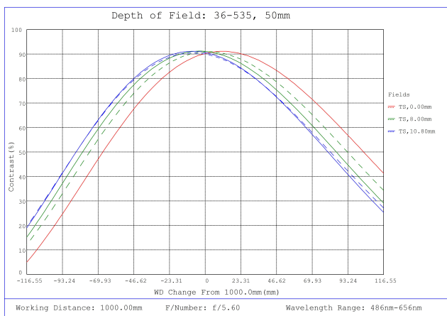
#36-535, 50mm f/5.6, HPr Series Fixed Focal Length Lens, Depth of Field Plot, 1000mm Working Distance, f5.6
