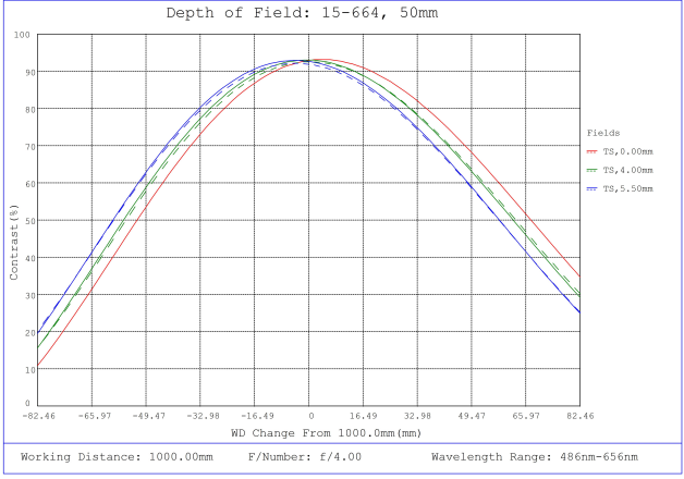
#15-664, 50mm, f/4.0 Sealed Cw Series Fixed Focal Length Lens, Depth of Field Plot, 1000mm Working Distance, f4
