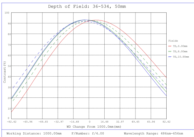
#36-534, 50mm f/4.0, HPr Series Fixed Focal Length Lens, Depth of Field Plot, 1000mm Working Distance, f4
