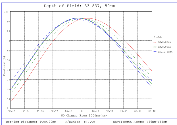
#33-837, 50mm f/4.0, HPI Series Fixed Focal Length Lens, Depth of Field Plot, 1000mm Working Distance, f4
