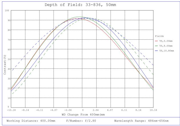
#33-836, 50mm f/2.8, HPI Series Fixed Focal Length Lens, Depth of Field Plot, 400mm Working Distance, f2.8
