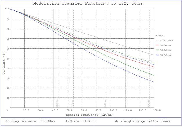
#35-192, 50mm, f/4.0 Cr Series Fixed Focal Length Lens, Modulated Transfer Function (MTF) Plot, 500mm Working Distance, f4
