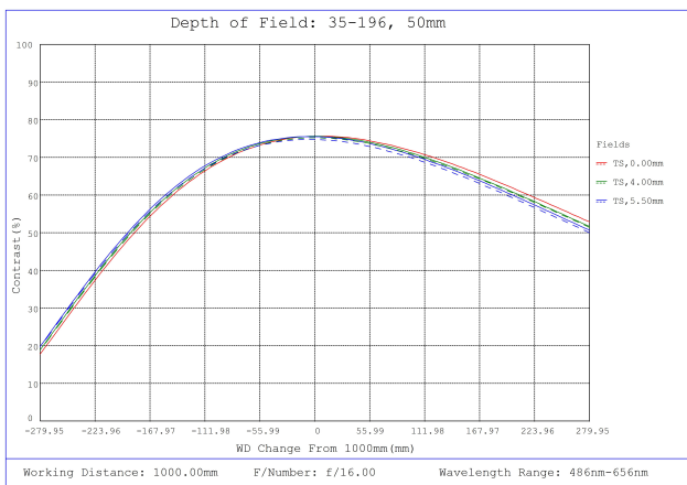
#35-196, 50mm, f/16 Cr Series Fixed Focal Length Lens, Depth of Field Plot, 1000mm Working Distance, f16
