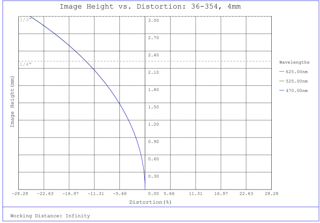
#36-354, 4mm FL f/5.6, Rugged Blue Series M12 Lens, Distortion Plot
