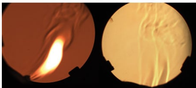
Flame Analysis using 6" Schlieren System
