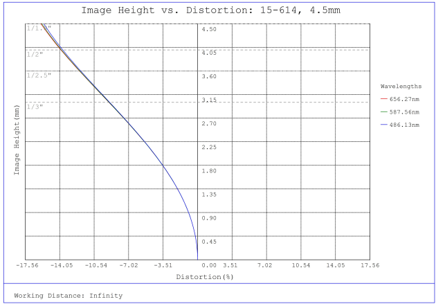
#15-614, 4.5mm f/2.8 Sealed Cw Series Fixed Focal Length Lens, Distortion Plot
