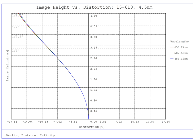
#15-613, 4.5mm f/2.0 Sealed Cw Series Fixed Focal Length Lens, Distortion Plot
