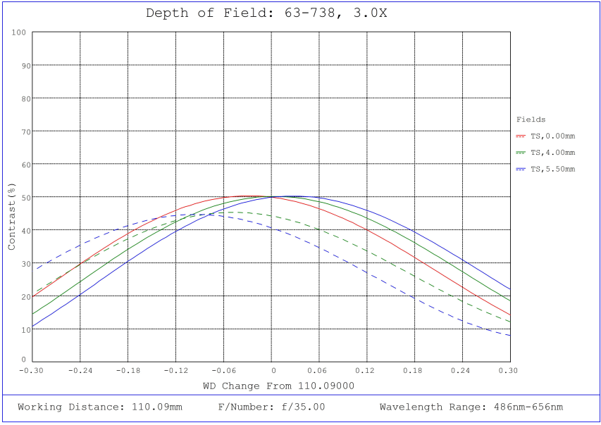
#63-738, 3X, 110mm WD CompactTL™ Telecentric Lens , Depth of Field Plot, 110mm Working Distance, f35
