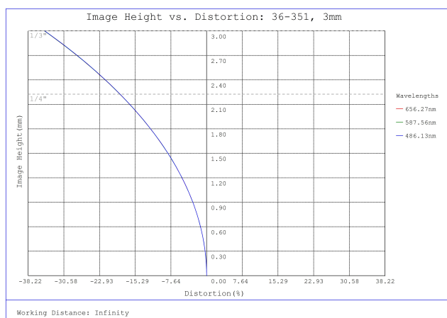
#36-351, 3mm FL f /8, Rugged Blue Series M12 Lens, Distortion Plot
