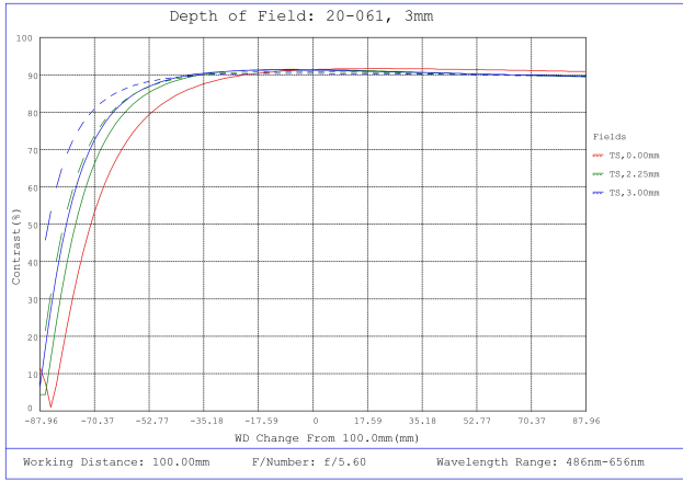
#20-061, 3mm FL f/5.6 IR-Cut Rugged Blue Series M12 Lens, Depth of Field Plot, 100mm Working Distance, f5.6
