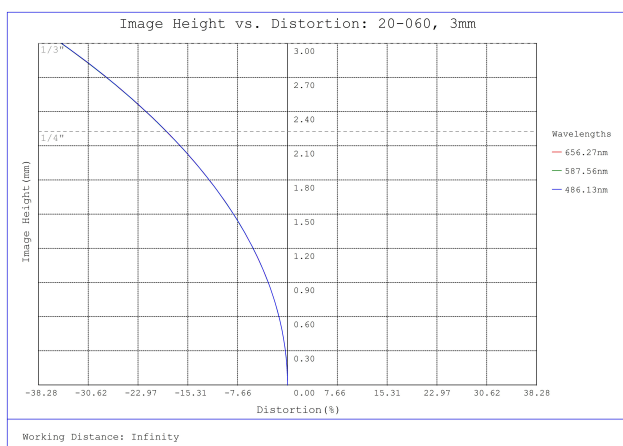
#20-060, 3mm FL f /4.0 IR-Cut Rugged Blue Series M12 Lens, Distortion Plot
