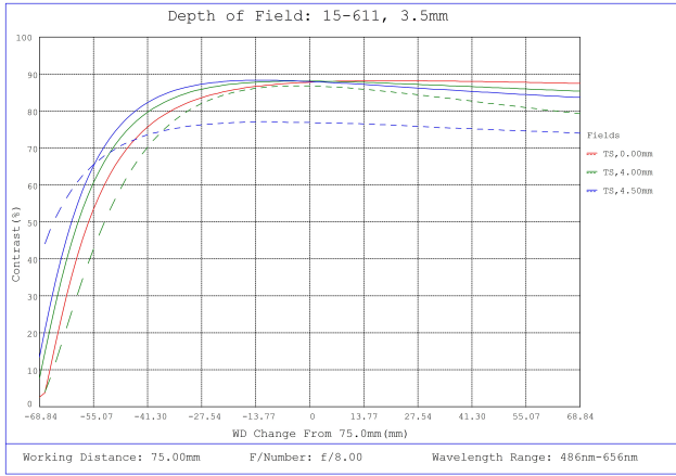
#15-611, 3.5mm f/8.0 Sealed Cw Series Fixed Focal Length Lens, Depth of Field Plot, 75mm Working Distance, f8
