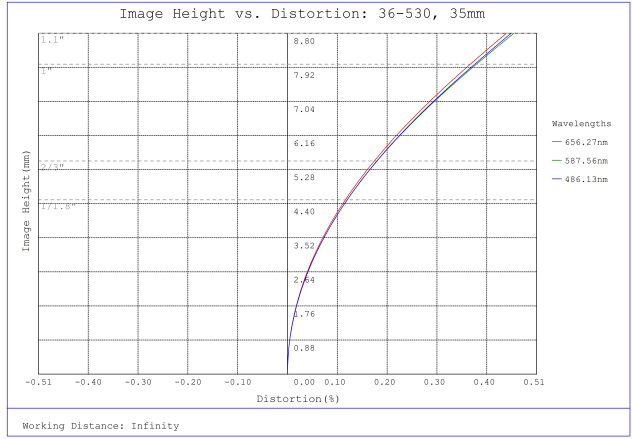
#36-530, 35mm f/8.0, HPr Series Fixed Focal Length Lens, Distortion Plot
