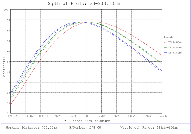
#33-833, 35mm f/8.0, HPi Series Fixed Focal Length Lens, Depth of Field Plot, 750mm Working Distance, f8
