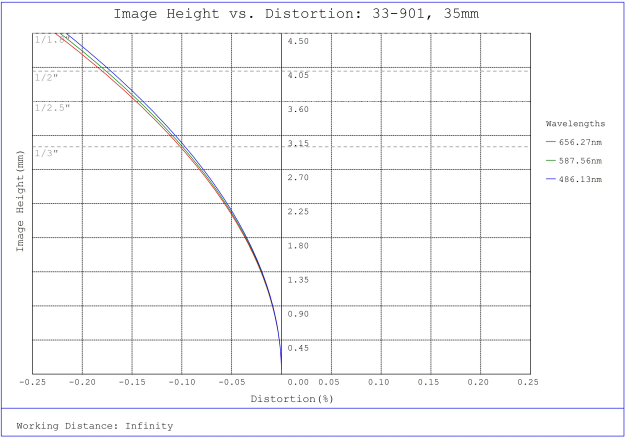
#33-901, 35mm f/8, UCi Series Fixed Focal Length Lens, Distortion Plot
