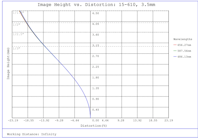
#15-610, 3.5mm f/5.6 Sealed Cw Series Fixed Focal Length Lens, Distortion Plot
