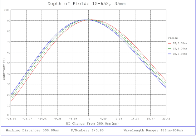
#15-658, 35mm, f/5.6 Cw Series Fixed Focal Length Lens, Depth of Field Plot, 300mm Working Distance, f5.6
