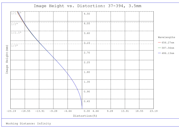
#37-394, 3.5mm, f/4 Cr Series Fixed Focal Length Lens, Distortion Plot
