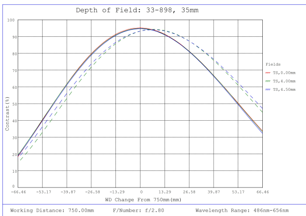
#33-898, 35mm f/2.8, UCI Series Fixed Focal Length Lens, Depth of Field Plot, 750mm Working Distance, f2.8
