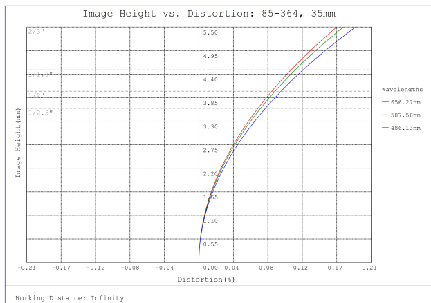
#85-364, 35mm, f/2.8 Ci Series Fixed Focal Length Lens, Distortion Plot
