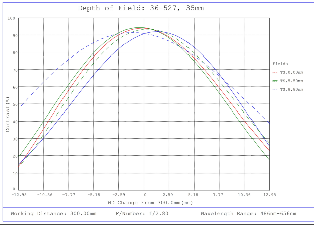
#36-527, 35mm f/2.8, HPr Series Fixed Focal Length Lens, Depth of Field Plot, 300mm Working Distance, f2.8
