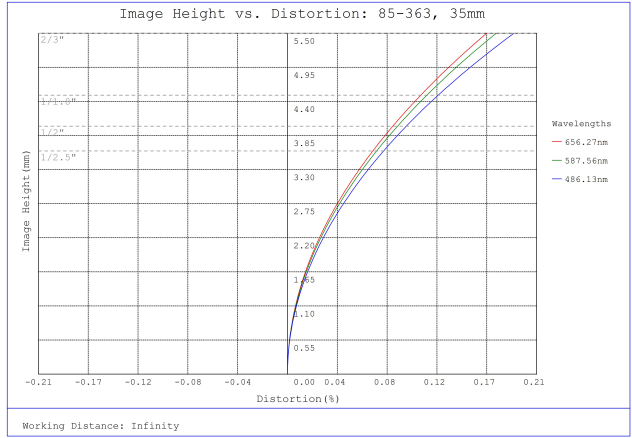
#85-363, 35mm, f/1.8 Ci Series Fixed Focal Length Lens, Distortion Plot
