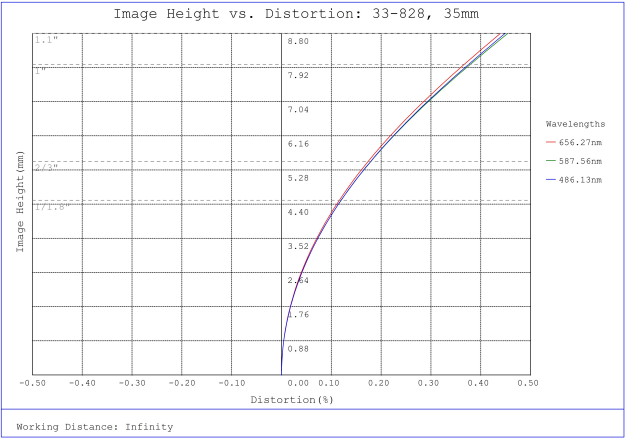
#33-828, 35mm f/1.8, HPi Series Fixed Focal Length Lens, Distortion Plot
