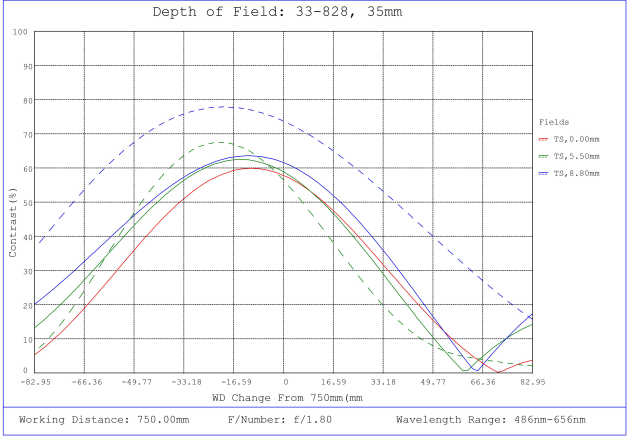
#33-828, 35mm f/1.8, HPi Series Fixed Focal Length Lens, Depth of Field Plot, 750mm Working Distance, f1.8
