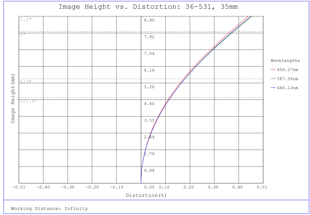
#36-531, 35mm f/11.0, HPr Series Fixed Focal Length Lens, Distortion Plot
