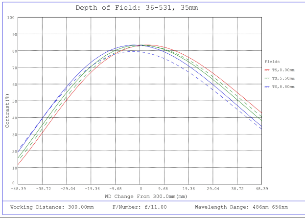
#36-531, 35mm f/11.0, HPr Series Fixed Focal Length Lens, Depth of Field Plot, 300mm Working Distance, f11
