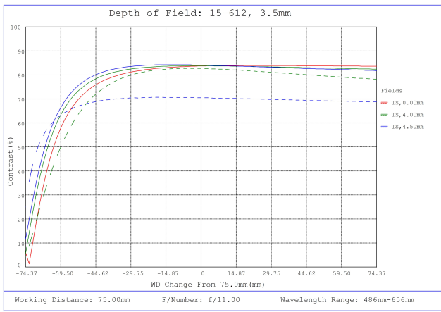
#15-612, 3.5mm f/11 Sealed Cw Series Fixed Focal Length Lens, Depth of Field Plot, 75mm Working Distance, f11
