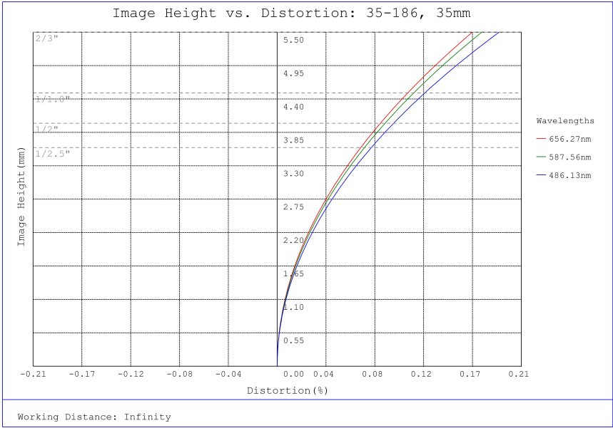
#35-186, 35mm, f/8.0 Cr Series Fixed Focal Length Lens, Distortion Plot
