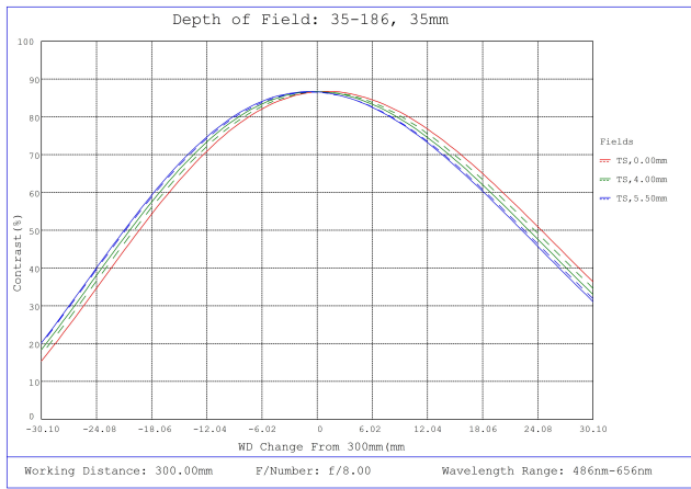
#35-186, 35mm, f/8.0 Cr Series Fixed Focal Length Lens, Depth of Field Plot, 300mm Working Distance, f8
