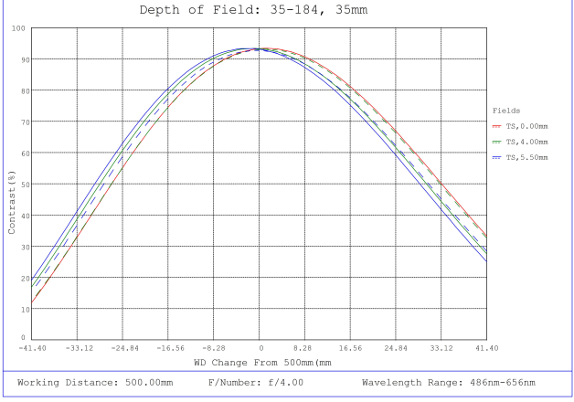
#35-184, 35mm, f/4.0 Cr Series Fixed Focal Length Lens, Depth of Field Plot, 500mm Working Distance, f4
