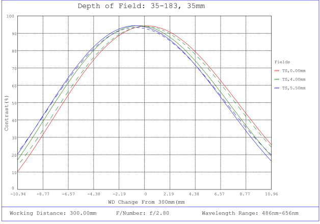
#35-183, 35mm, f/2.8 Cr Series Fixed Focal Length Lens, Depth of Field Plot, 300mm Working Distance, f2.8
