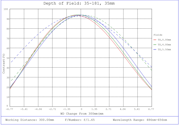
#35-181, 35mm, f/1.65 Cr Series Fixed Focal Length Lens, Depth of Field Plot, 300mm Working Distance, f1.6
