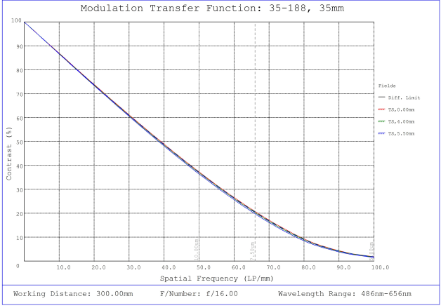
#35-188, 35mm, f/16 Cr Series Fixed Focal Length Lens, Modulated Transfer Function (MTF) Plot, 300mm Working Distance, f16
