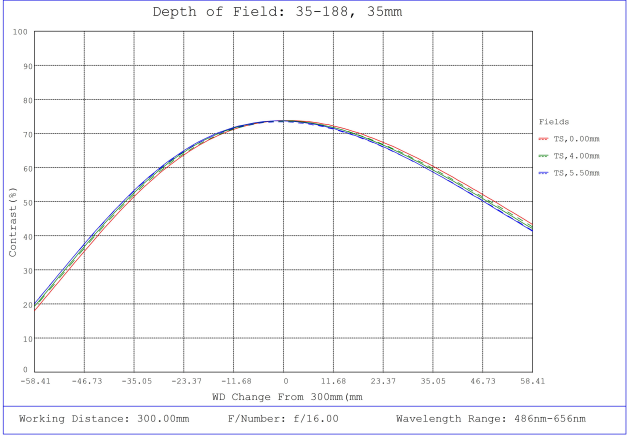
#35-188, 35mm, f/16 Cr Series Fixed Focal Length Lens, Depth of Field Plot, 300mm Working Distance, f16
