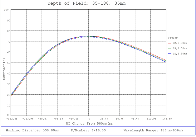
#35-188, 35mm, f/16 Cr Series Fixed Focal Length Lens, Depth of Field Plot, 500mm Working Distance, f16
