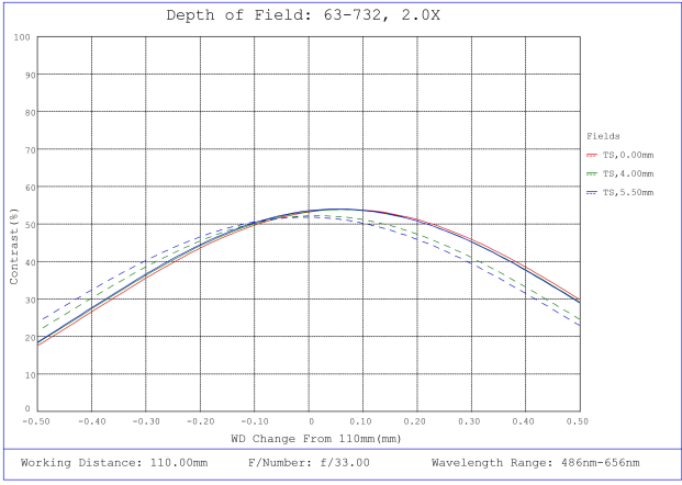
#63-732, 2X, 110mm WD CompactTL™ Telecentric Lens, Depth of Field Plot, 110mm Working Distance, f33
