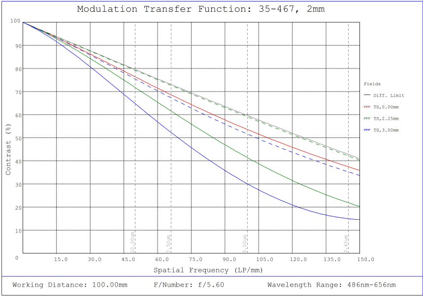
#35-467, 2mm FL f/5.6 IR-Cut, Blue Series M12 Lens, Modulated Transfer Function (MTF) Plot, 100mm Working Distance, f5.6
