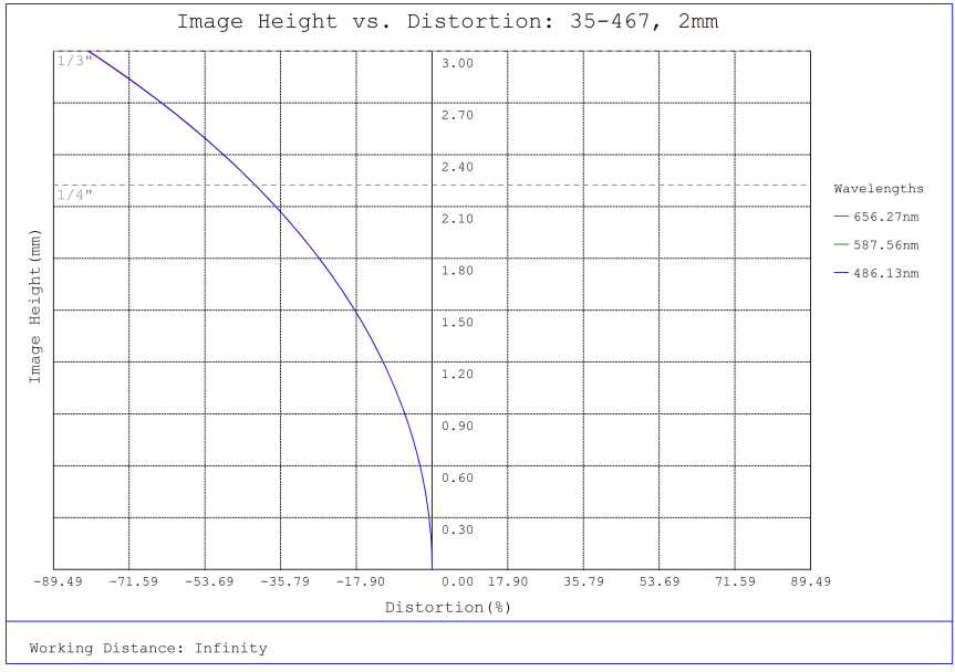
#35-467, 2mm FL f/5.6 IR-Cut, Blue Series M12 Lens, Distortion Plot
