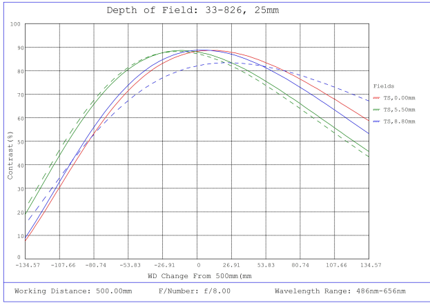
#33-826, 25mm f/8.0, HPI Series Fixed Focal Length Lens, Depth of Field Plot, 500mm Working Distance, f8
